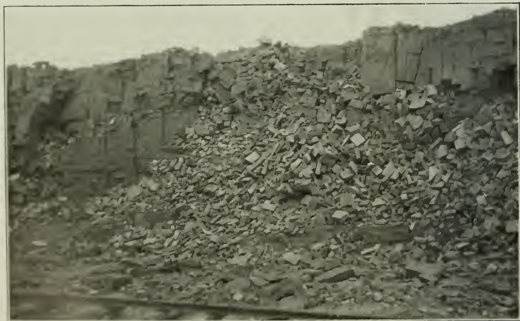
Open Cut Ore Face, showing Characteristic Rhombohedral Cleavage, at Wabana Iron Mines.
